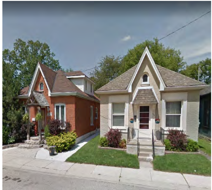
Front entrances should front the street and be fully visible, located at a height of approximately 1.5 metres above grade / Chestnut Ave.
