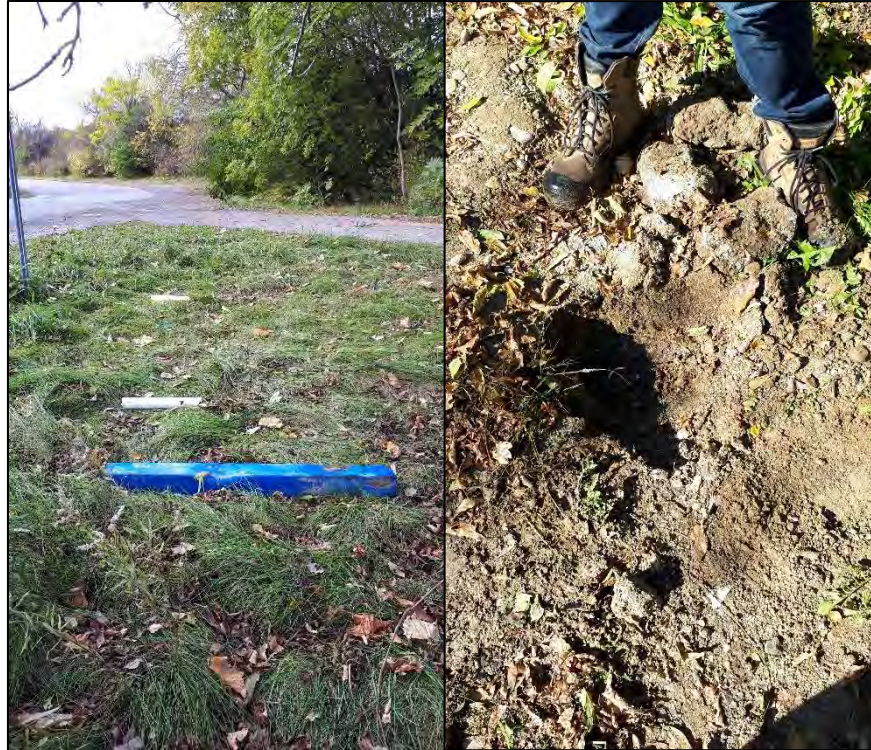
Figure 5.27: Condition of BH/MW-5 after collision (Pictures taken October 23, 2018)
