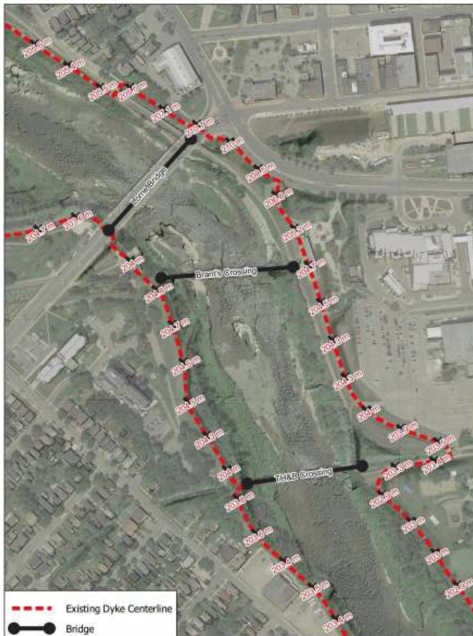
Figure 5. Existing Brantford Dykes Alignment and Elevations
